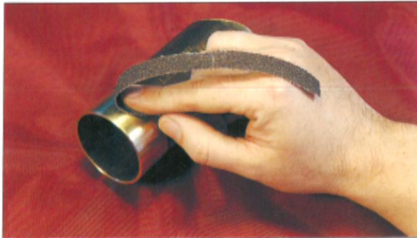
C - Clean outside of tube with emery cloth
