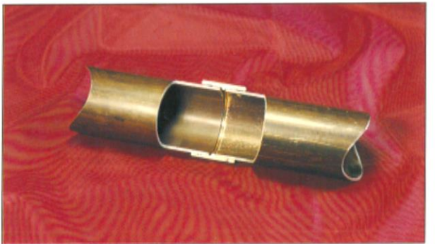
H - Pipe and fitting correctly lined up
