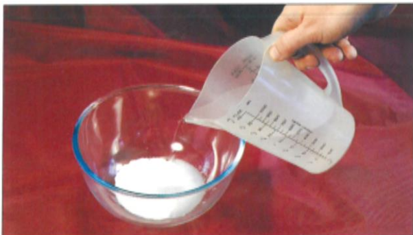
E - Add water to powder flux
