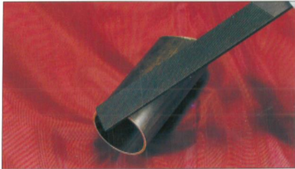
A - Remove burr inside and outside
